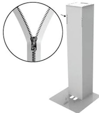
Once the scrim has been applied unzip each zipper to mount the TV bracket.
