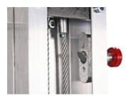
Safety pins: Allow selecting different heigths and spreading the load to all bars equally.
