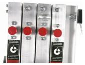
**Safety pins:** Safety pins avoid the load from falling. Besides, they allow selecting different heights, raising all bars equally and distributing the load from the mast to the last bar, which extends the tower's lifetime and increases its stability.
