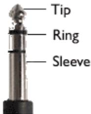
**TRS** is the abbreviation for "Tip, Ring, Sleeve." It looks like a standard 1/4" or 1/8" plug but with an extra "ring" on its shaft. TRS cables have two conductors plus a ground (shield). They are commonly used to connect balanced equipment or for running both left and right mono signals to stereo headphones. You will also find TRS connectors on the stem of Y cables. These are used for mixer insert jacks where the signal is sent out through one wire and comes back in through the other.
