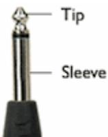
**TS** is the abbreviation for "Tip, Sleeve" and refers to a specific type of 1/4" or 1/8" connector that is set up for 2-conductor, unbalanced operation. One insulator ring separates the tip and sleeve. The tip is generally considered the "hot," or the carrier of the signal, while the sleeve is where the ground or shield is connected. TS cables are best known as guitar or line-level instrument cables.
