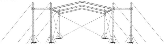
Pre-Designed Truss Packages: The sunshade style (pictured above) has been a long time favorite of the touring industry and now with smaller designs is quickly becoming a favorite layout for small to medium sized production needs. With the ability to have rapid assembly, disassembly and easy transport, the Sunshade can be obtained in several pre-designed packages which can be utilized in a variety of locations. More importantly,
