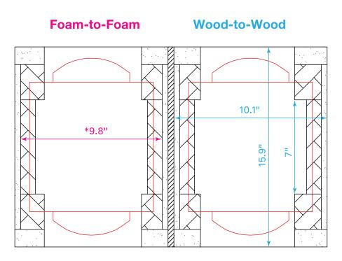
\*Foam inserts can be removed or modified to extact area of the wood edges.
